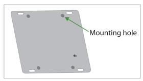
Distance between the enclosure mounting holes: 42.00 x 62.53mm
