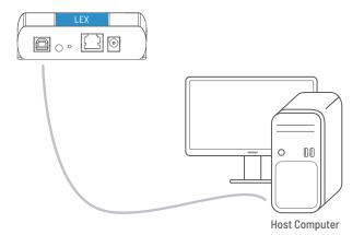
2 Connect a CAT 5e/6/7 patch cable from the RJ45 Link port on the LEX to an IEEE 802.3at - PoE+ (25.5W) capable LAN port.
